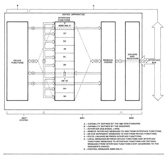
Figure D.1. Functional Partition Within a Device.
